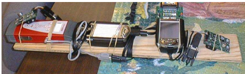
Figure 3: A prototype “software marker” (a software compass integrated with a laser range-finder).
