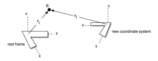
Figure 3-4: When the frame is moved, it creates a new coordinate system. The vector to beacon B in one coordinate system,  $\mathbf{r}_r$ , is not equal to the vector to B in the other coordinate system,  $\mathbf{r}_l$ .
