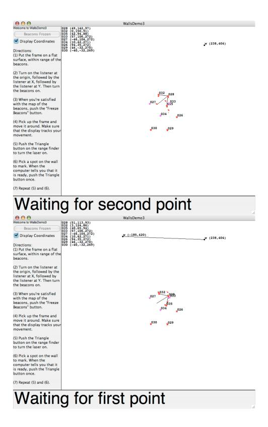
Figure 3-10: Two screenshots of WallsDemo3, showing a user marking out walls on the same map with beacon positions. (Above) The user has marked one wall vertex, and the software is waiting for the second vertex of the pair. (Below) The user has marked the second wall vertex, and the software has drawn the line of the corresponding wall.
