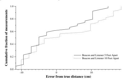
Figure 2-4: CDF of distance measurements between a Version 1 listener and beacon at 5 feet and 10 feet.
