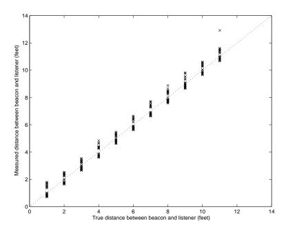
Figure 2-3: Scatterplot of distance measurements between a Version 1 listener and beacon at various separations. The dashed line represents where ideal measurements would lie.
