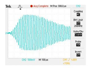
Figure 2-9: The figure on the left shows the ultrasound pulse "envelope," as measured after the cricket listener's amplification stage, but before rectification. The figure on the right shows a closer view of the same signal, so it is easier to see the main 40 kHz signal.
