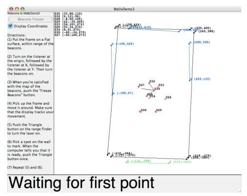
Figure 3-11: Screenshot of WallsDemo3 after creating a map of 32-D451. In this example, the frame was tracked using three beacon trilateration.
