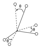
Figure 3-7: Once the two planes are aligned, points in the left hand plane must be rotated by  $\theta$  radians to minimize the sum of the squared error between pairs of measurements. In a transformation with no measurement error, the points will align perfectly.
