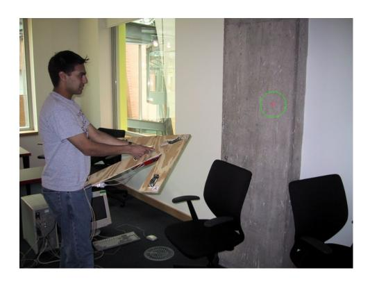
Figure 3-9: A user marks a wall vertex using the frame and range finder. The range finder projects a red spot on the wall (shown here circled in green), which indicates to the user which feature s/he is about to mark.
