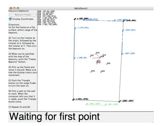
Figure 3-12: Screenshot of WallsDemo3 after creating a map of 32-D451. In this example, the frame was tracked using Horn's coordinate transformation algorithm. The improvement in accuracy is primarily because Horn's algorithm constrains the three frame listeners to be localized in a rigid orientation.
